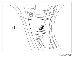
Use this stowage to keep small articles. You can open the lid (1) by pressing the raised portion on it.
